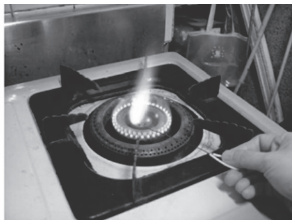
Picture 41. Beilstein Method with oil in a copper wire
