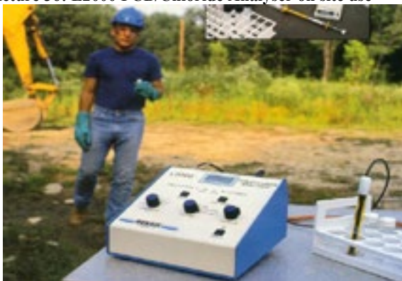
Picture 36: L2000 PCB/Chloride Analyser on site use
