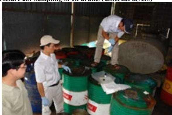
Picture 25: Sampling of oil drums (different layers)
