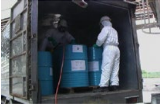
Emptying PCB drums for trial burn
