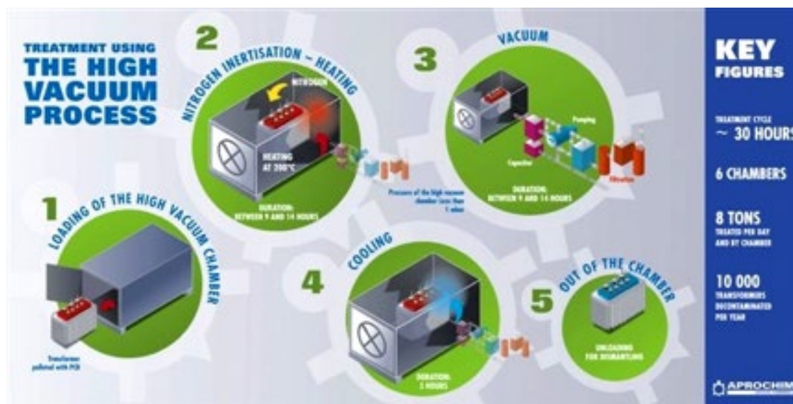
Figure 3: High vacuum process adapted for materials contaminated by PCBs
