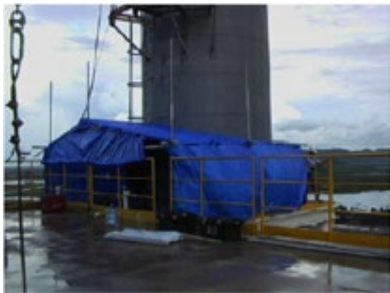
Emission testing facility on kiln stack
