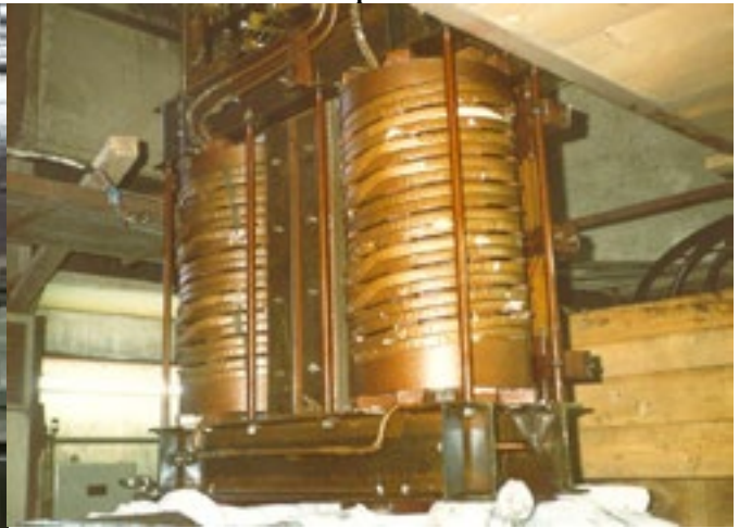
Picture 40: Active transformer part in service station
