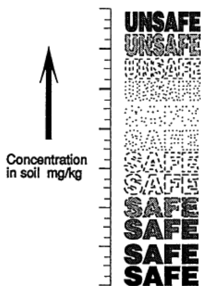
Figure 2. Schematic illustration of 'safe' and 'unsafe' zones separated by a diffuse boundary zone.
