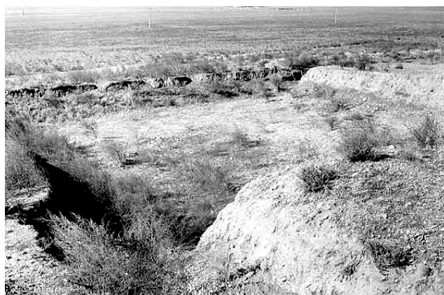
Photo 2: Soil subsidence as a result of sharp phreatic rise at the site of pesticides burial
