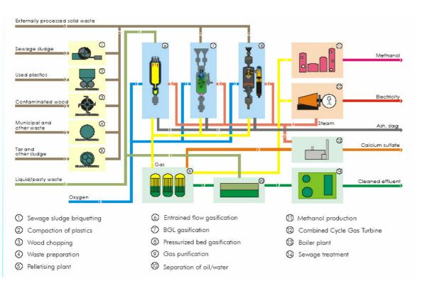
SVZ operated a complex plant system for producing highly pure synthesis gas from hydrocarbon-containing waste and this system included downstream methanol production. Core units of the plant system were:
