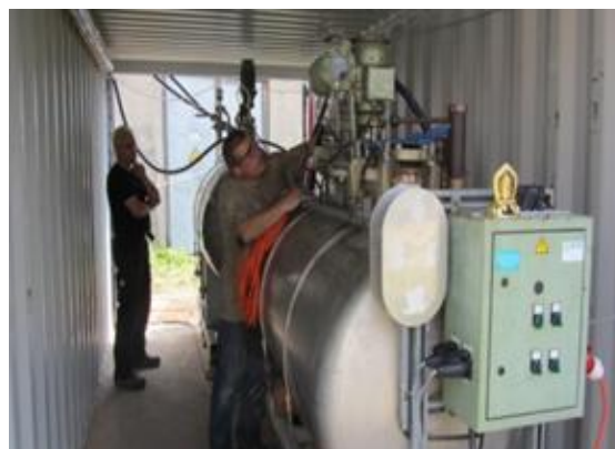
Photo 2: The apparatus for the elimination of the methyl bromide. Photo: W. Schimpf
