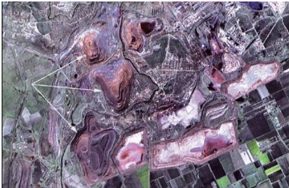
Ore processing tailings management facilities (Photo: Grigory Shmatkov)
