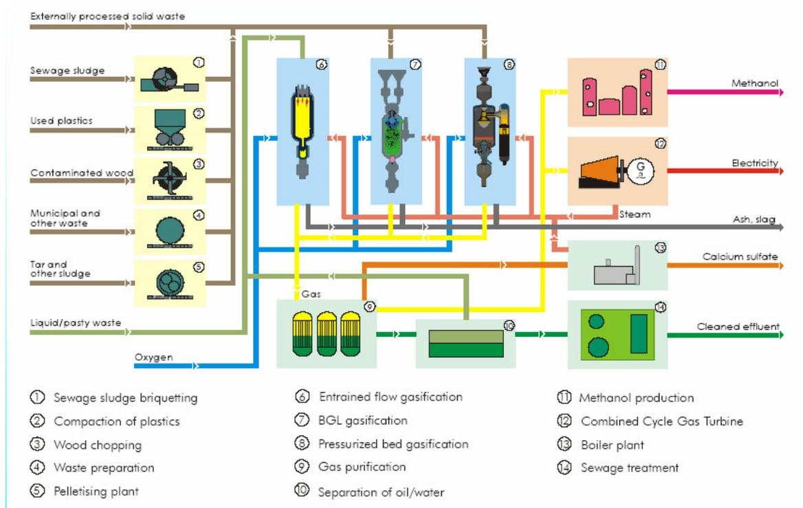
SVZ operated a complex plant system for producing highly pure synthesis gas from hydrocarbon-containing waste and this system included downstream methanol production. Core units of the plant system were:
