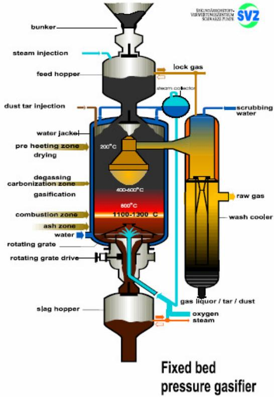
Figure 3: Slagging Gasifier BGL
